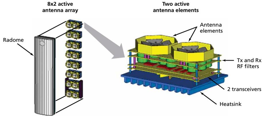
The lightRadio family significantly extends antenna technology using smart active antenna arrays (AAAs). This advance can obtain MIMO gains and allow sophisticated beamforming, so the RF energy can be dynamically directed exactly where needed, based on dynamic changes in cell loading and traffic density. Figure 9 illustrates one novel AAA design that is part of the lightRadio product family.
