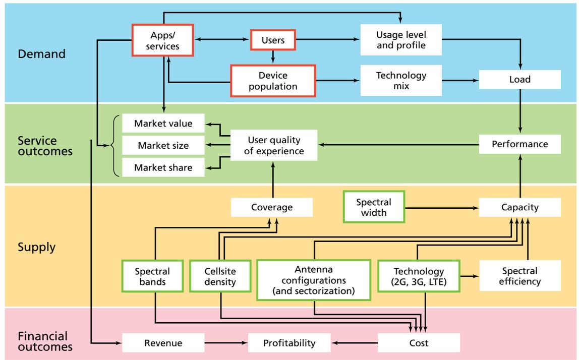
Five key supply factors optimized by the lightRadio paradigm are highlighted in Figure 3. These five factors directly impact network costs, so any architectural shift must seek to minimize costs, especially in key categories such as transmission, site rental, civil works, equipment, power, maintenance, repair and operations, which are shown in Figure 4.
