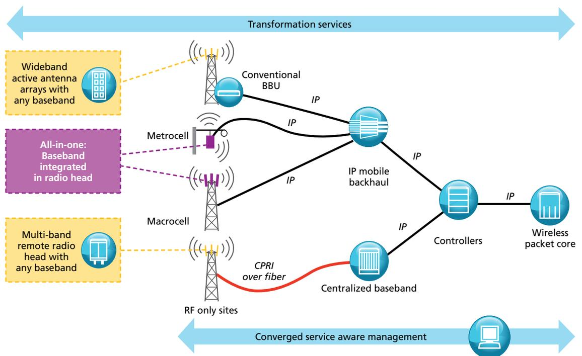
The five technology components of the lightRadio product family are also identified. They include antennas, radios, baseband, controllers and management. These elements collectively create the following five business enablers, which optimize capacity, coverage and performance:
